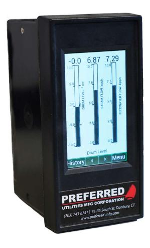
The **JC-43D2** 3-Element Drum Level Controller maintains a boilers drum level at setpoint by modulating a 4-20 mA control output with a user selectable 1-element, 2-element, or 3-element PID loop.
