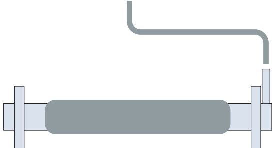
Double-walled Piping with Vacuum Leak Detector
