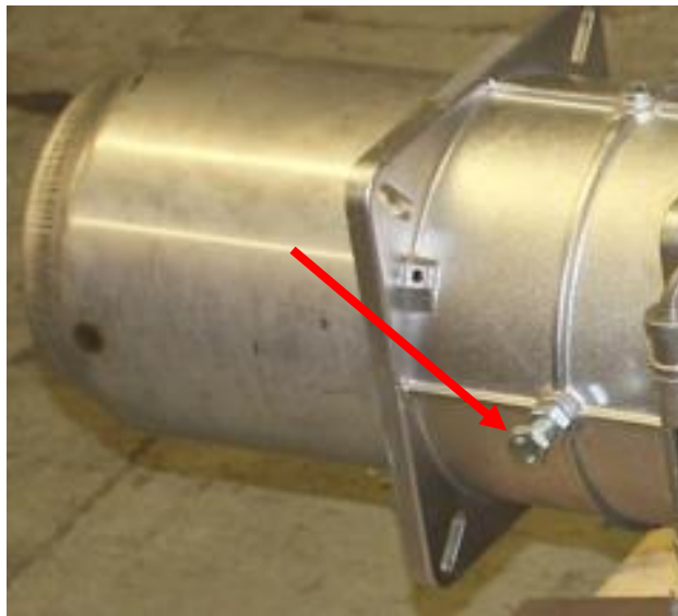
Bolt for Removing Burner Head Figure 10
